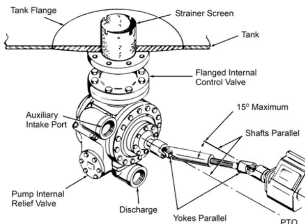
Note: A Drive Shaft Guard between the pump and the PTO MUST be provided. (Not Shown)
