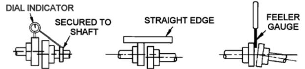
Figure 5 – Coupling Alignment
