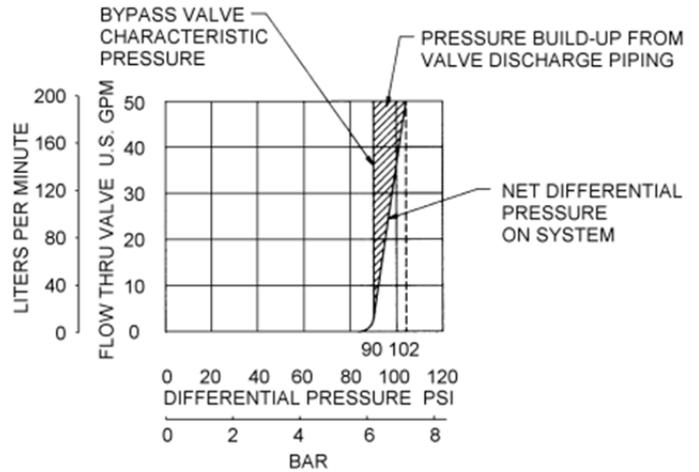
For example, the BV1.25A bypass valve has a characteristic pressure when set at 90 psi (6.21 bar) as shown on the following curve. If the friction loss through the bypass valve, discharge pipe and fittings (pipe, elbows, tees, shut-off valve, check valve, etc.) is 12 psi (.84 bar) at 50 gpm (189 lpm) flow rate, then the actual differential pressure in the system will rise under bypass conditions, as illustrated on the curve.
